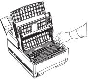
6. Once the toner cartridge is in place, push the colored lever all the way forward to secure it and release the toner.
